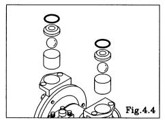
• Remove the O ring, valve seat, ball and valve stopper. [Fig.4.4]
