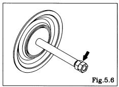
• Fix a double nut to one end of the center rod and take the diaphragm and center disk off the opposite end. [Fig.5.6] Be careful not to scratch or score the center rod.
