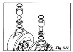
• Remove the O ring, valve stopper, ball and valve seat. [Fig.4.6]
